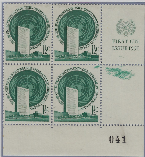
An ink smear resulted when the slip sheet inserted between printed sheets moved on the wet sheet.
